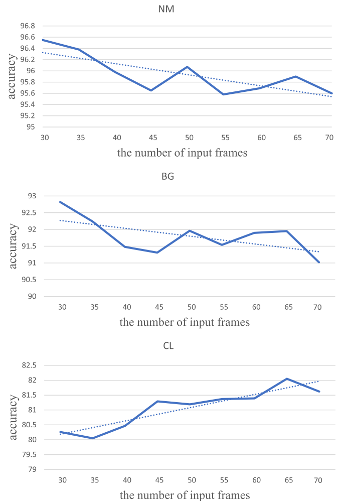
Fig. 7. The result when the number of input frames is different. Dotted lines show the trend of the data. More input frames can improve the accuracy under occlusion.
